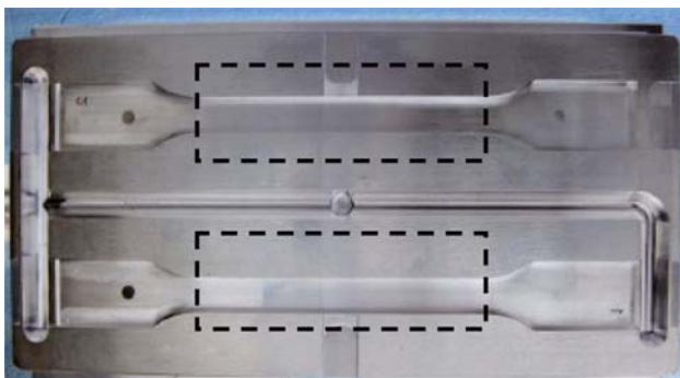
Fig. 1 Single- and double-gated cavities with nominal dimensions of 4 \times 10 \times 120 mm (thickness, width, length)
